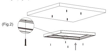
Step 5: Slide the LTSP70 Panel Light into the frame (Fig. 3)
